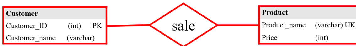
Figure 10 Physical model (PK: Primary key, UK: Unique Key)
